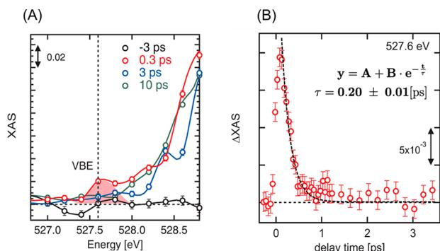
**Figure 2.** (A) Zoom of the pre-edge region shown as a dashed rectangle in Figure 1B. (B) Kinetic trace of XAS at 527.6 eV shown in Figure 1D. The dashed line is a single exponential function used for fitting.
