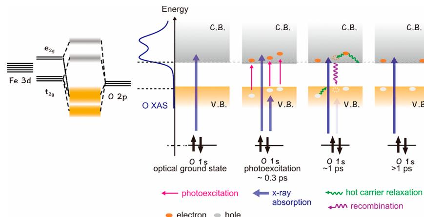
**Figure 3.** An illustration for the electronic state of the photoexcited  $\alpha\text{-Fe}_2\text{O}_3$  from the viewpoint of O K-edge XAS. The conduction band is denoted as C.B. and the valence band is as V.B.
