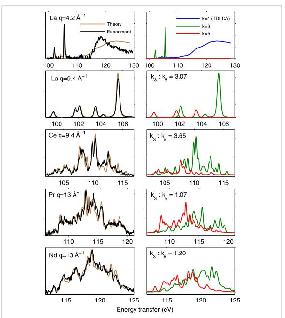
**Figure 6.** The  $4d \rightarrow 4f$  excitations, La to Nd. For La, two momentum transfer values are shown; for others, only a large momentum transfer setting was used in order to focus on the high-order multipolar transitions. Left panels: experiment and theory. Right panels: theory decomposed to different multipolar components (k = 1, 3, 5). The relative weights between the components k = 3 and k = 5 are indicated.
