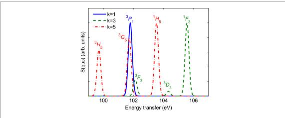
**Figure 3.** Different multipolar components of the spectra seen in figure 2. The spectra have been normalized to the maximum of each multipole spectrum.
