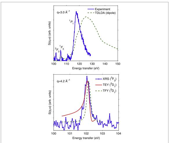
Figure 1. Upper panel: LaPO $_4$  4 $d \rightarrow 4f$  spectra, measured with 1-eV energy resolution. The giant dipole resonance dominates the experimental spectrum, with weak multipolar features (pre-resonances) at lower energies. The experimental result is compared with a TDLDA computation. Lower panel: the  $^3F_3$  peak seen closer with 180-meV resolution, to observe its inherent line shape, compared with the dipolar  $^3D_1$  peak measured with TEY and TFY XAS (taken from [1]).
