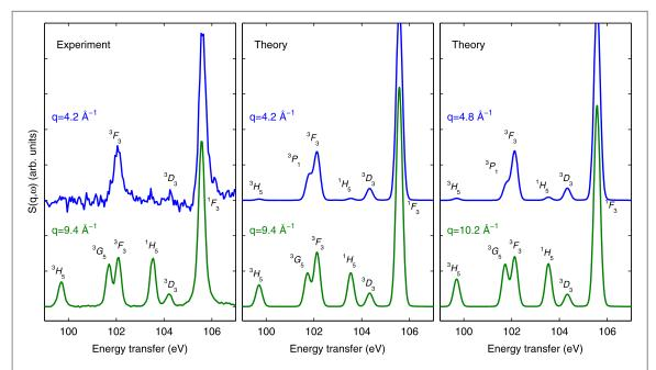
**Figure 2.** La  $4d \rightarrow 4f$  pre-resonance region of LaPO<sub>4</sub> measured with 180-meV resolution. Also shown are atomic multiplet theory results for the experimental momentum transfer and for a higher momentum transfer that fits the experimental result better.
