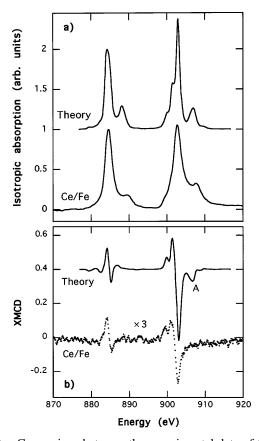
FIG. 3. Comparison between the experimental data of the Ce/ Fe multilayer and the results of the model described in the text. Top panel, Ce- $M_{4,5}$  isotropic spectra; lower panel, XMCD spectra. The intensity of the two  $M_5$  edge isotropic spectra has been set to unity. The origin of the energy axis of the theoretical spectra has been chosen in order to align the positive peaks at correspondence with the  $M_5$  edge of the theoretical and experimental XMCD spectra.
