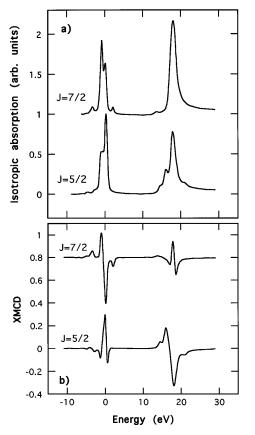
FIG. 2. Ce- $M_{4,5}$  isotropic (top panel) and XMCD (lower panel) spectra obtained for the  $J = \frac{5}{2}$  and  $J = \frac{7}{2}$  states calculated for the ion Ce<sup>3+</sup>. The zero of the energy axis has been chosen at correspondence with the maximum in the  $M_5$  edge of the  $J = \frac{5}{2}$  XMCD spectrum. The intensity of the  $M_5$  edge of the  $J = \frac{5}{2}$  isotropic spectrum has been set to unity.
