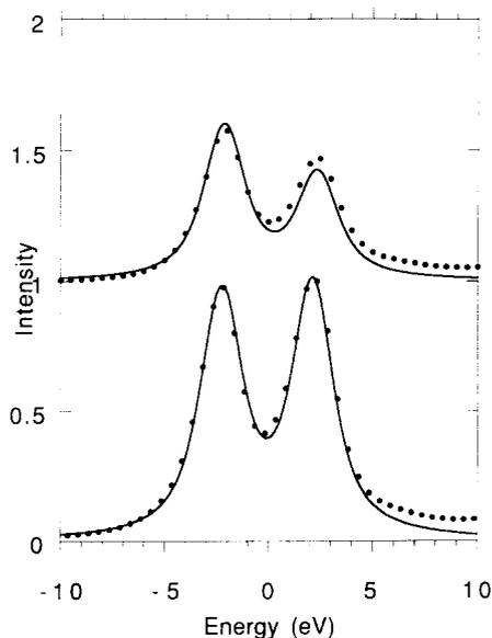
Fig. 1. Comparison of a crystal field multiplet calculation of Mo<sup>6+</sup>, 4d<sup>0</sup> (solid line) with an experimental spectrum of gas-phase MoF<sub>6</sub> (points). The L<sub>2</sub> edge (top) and the L<sub>3</sub> edge (bottom) have been aligned. A crystal field strength of 4.5 eV was used.
